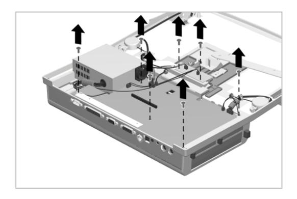
Figure 6-17. Removing the Main Board Screws
